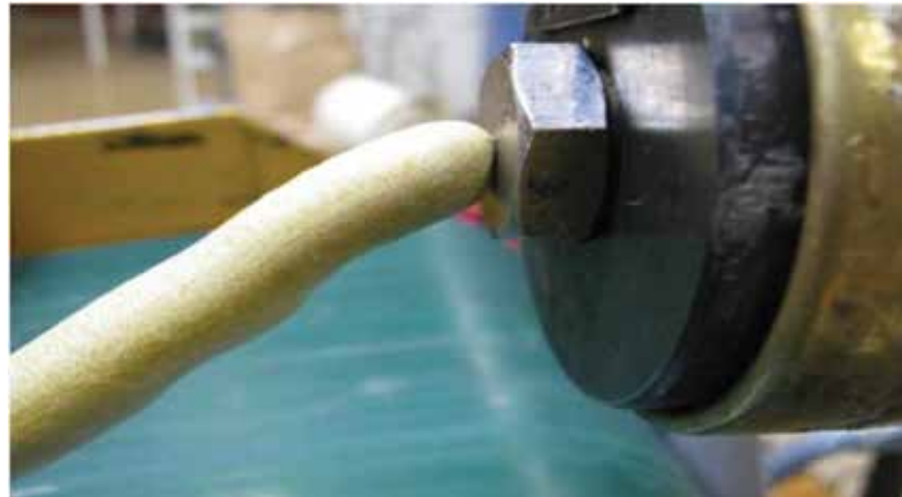
Figure 3. Extrusion foaming of the zein-pearl millet flour blend.
