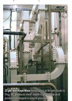
thermal processing systems with a built-in, extensively and robustly tested scale-up strategy and controllability at pilot plant (2–4 gal/min), intermediate (10–20 gal/min), and high (20–40 gal/min) industrial throughput levels. The technology provides virtually instantaneous and tightly controlled thermal come-up and rapid cool down, minimizing product losses in changeovers and shutdowns for cleaning in place.
