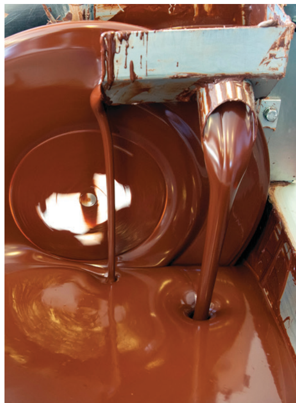
Rollers produce a smooth emulsion during the conching phase of chocolate processing. © IMNATURE/iStock/Thinkstock
