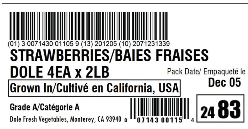
Figure 9. Harmonized PTI Label, illustrating the use of Application Identifiers in the GS1-128 barcode.
