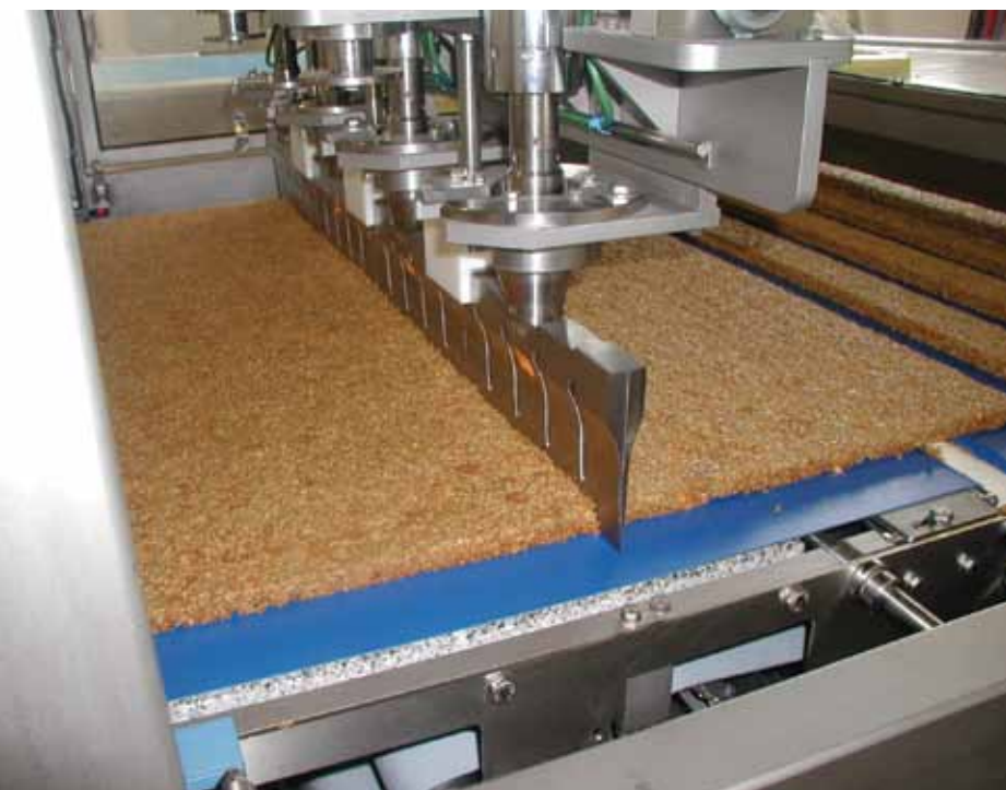
A bank of Branson Ultrasonics horns slicing granola. Photo courtesy of Branson Ultrasonics Corp.
