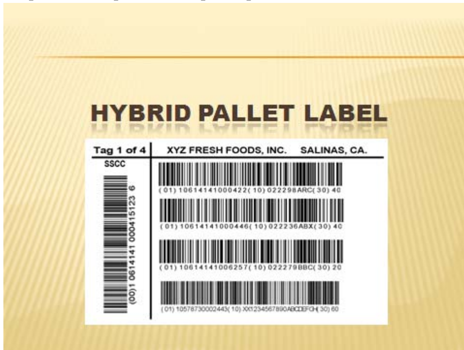
Figure 5. Example of a hybrid pallet label that communicates how many cases of each lot are present on a pallet, developed as part of the PTI (Produce Traceability Initiative).
